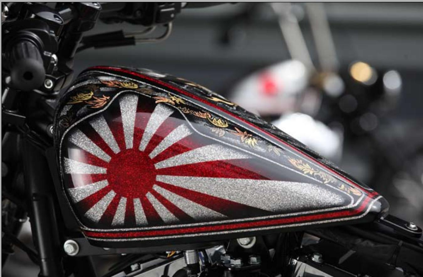
**TOP:** W&W Cycles fuel tank with flush-mounted Tolle fuel cap, modified by the Baechli sheet metal workshop. To mount the small tank to the stock Softail fuel injection – and keep it invisible under the tank – the Sportster fuel pump was used.
