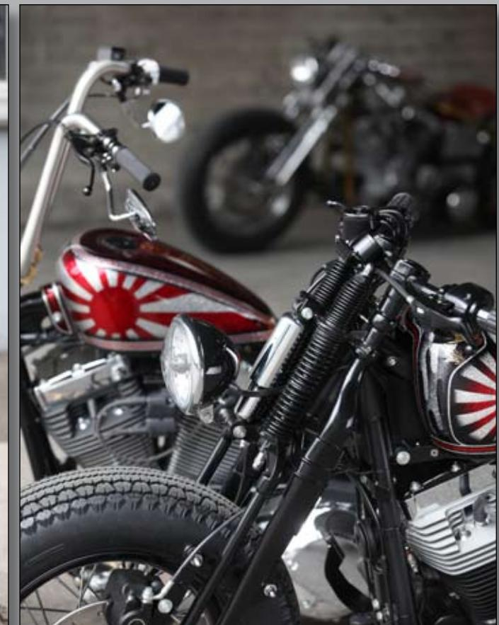
**TOP RIGHT:** W&W Cycles Springer fork and low mounted CCE headlight compensate for the missing „Gooseneck“ frame
